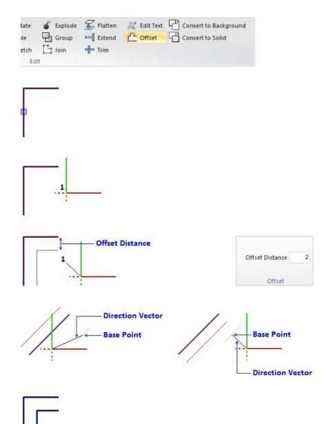
For multi-segment **Background Objects**, the behavior of the direction *vector* is often non-*linear* and complex as can be seen at right. It is recommended that the implied *drawing* feature inherent to the command be used to determine if the **Offset** is desirable and/or where the **Offset** object will be created.
